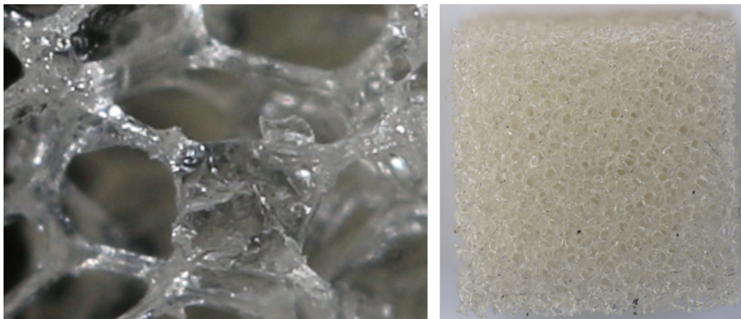
Figure 8 Barren collection media post stripping and washing, close up on the left and a 12.5mm media cube on the right
