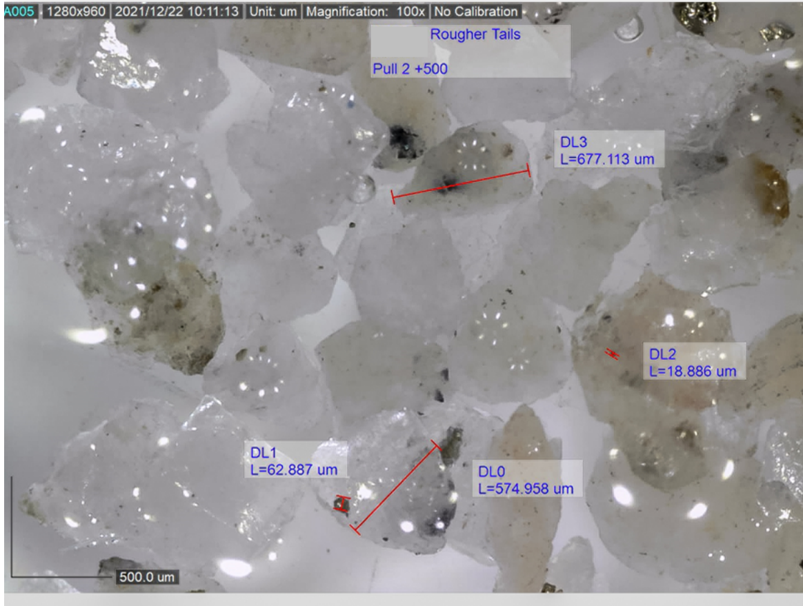
Figure 9 P29 concentrate from scavenging rougher tailings at a size fraction of +500µm
