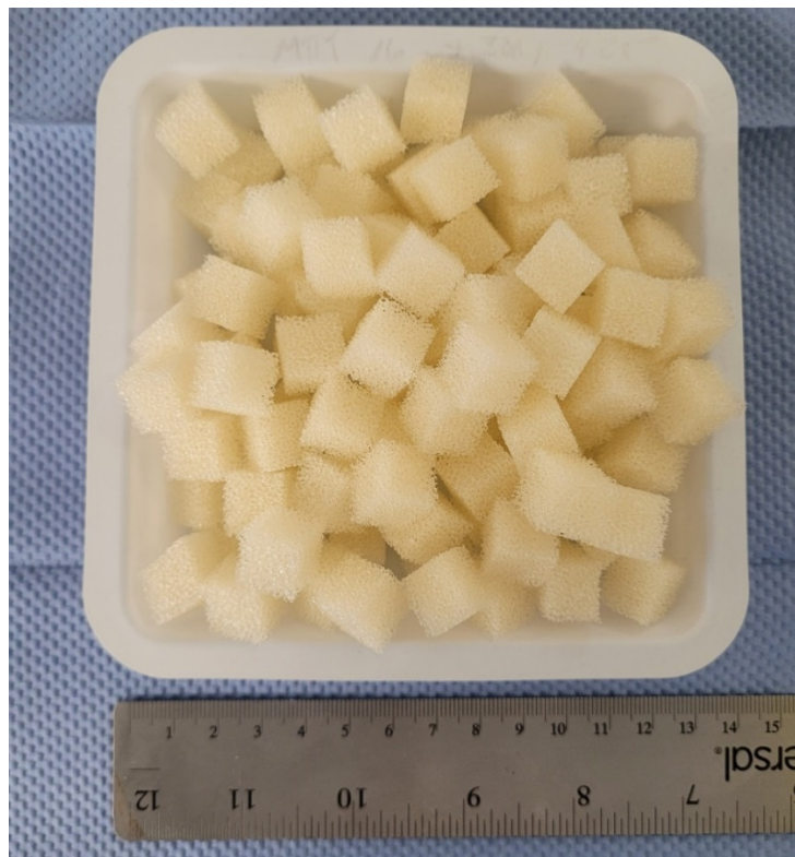
Figure 12 P29 polymer coated collection foam media at 12.5mm x 12.5mm x 12.5mm
